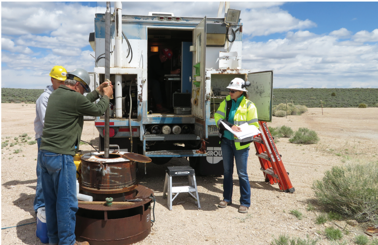
NNSS Scientists collect water samples at Well ER-20-1, a 2,065 feet deep early detection well on Pahute Mesa in 2019.
